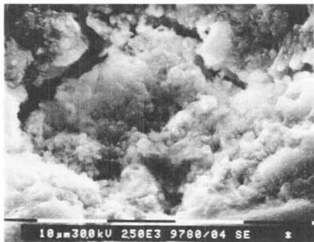
Figure 4: Inner pore space of a cementitious product; w/c ratio 0.34; CsNO 3 50 g/l.
