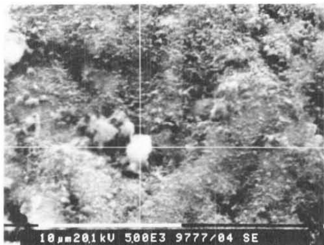
Figure 5: Globular CsNO 3 precipitation in the pore space matrix.
